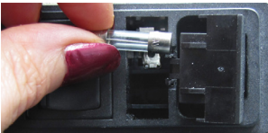
Fig. 12—Open the fuse housing and rotate it right to remove the fuse.
